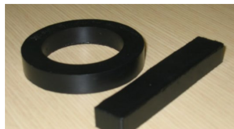
Washer and Bar Shrinkage Mold Samples
