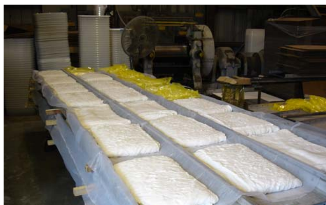
FIGURE 2: PREMILLED MILLATHANE 76 MILLED SHEETS
